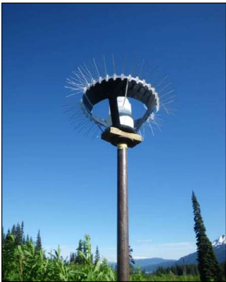
Plate 1. Dustfall container inside wind shield housing. Plate 2. Typical dustfall collection site.
